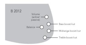
Addition passive tone control available as a single shaft pot or as a concentric pot with active treble control.
